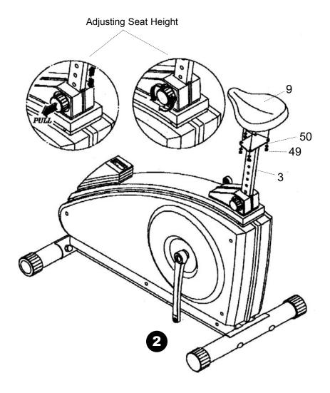
**2.** Attach the seat (9) to the seat post (3) with the locknuts (49) and flat washers (50) already provided on the underside seat bolts.
